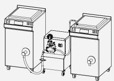
When the product in the first pasteurizer reaches the pasteurization temperature of 85-90°C, then the homogenizer transfers the product into the second pasteurizer to accomplish the cooling duty.
