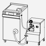
Once the product in the pasteurizer reaches the temperature of 50°C and the sugar has been fully solubilized, the homogenizer starts recirculating the batch in a loop (5 times approx), to make sure the ice cream is fully homogenized.
